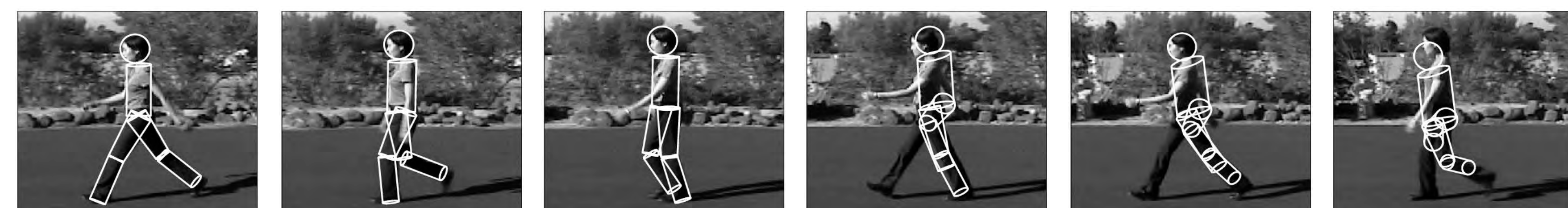
Every 4th frame of lower body tracking with the Particle filter, N = 20,000 samples.
